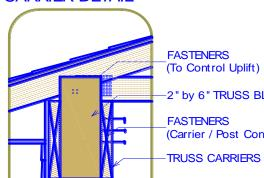
Truss Blocking to Truss connection can be calculated by dividing the shear strength of the fastener and the design uplift from the Truss Specs. (16d fasteners have a design shear strength of 101 lbs per nail)
